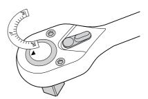
To use the angle scale, point the arrow on 0°. Put the wrench on the nut/ screw and thoroughly register where the handle is located. Turn the wrench to estimated angle, then return the wrench to the starting position. Now the turned angle can be read.
